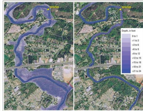
Figure 1. U.S. Geological Survey (USGS) flood-inundation maps for a 3.95-mile reach of the Saluda River near Greenville, South Carolina, originating approximately 150 feet downstream from Saluda Lake Dam. A lidar-derived digital elevation model was used to aid in hydraulic modeling to create these maps. The extent of inundation depicted corresponds to river stages of 20.0 feet (A) and 6.0 feet (B) at USGS streamgage 02162500 (yellow triangle) on the Saluda River. The red line corresponds to the model extent.
