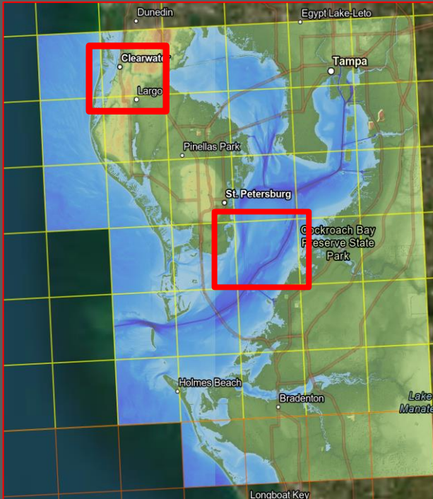
Composite of sources based on topobathy lidar and traditional acoustic sonar technologies
