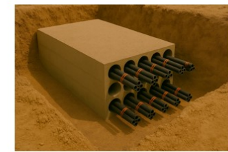
Common Duct Network (Telco)
