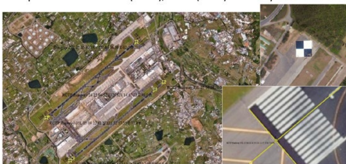
Figure 13 Example 3D geolocation testing at Taipei International Airport, Taiwan using Maxar’s Precision3D DSM and TrueOrtho imagery and airport runway markers for DGPS reference with a measured absolute accuracy of CE90 of 0.7m and LE90 of 1.1m (left and lower). The inset image (upper right) is the knife edge calibration target at Punghu Airport (23.519989 N 119.583726 E).
