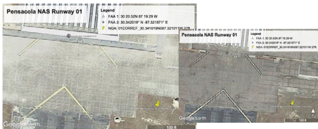
Figure 10 Two examples of a runway in 2020 (left) and 2016 (right) illustrating typical maintenance differences at airfields that confound data fusion and registration.
