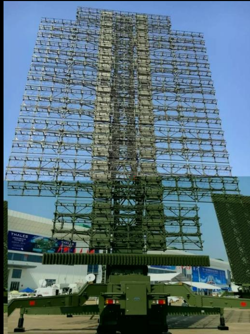
JY-27A ANTI STEALTH RADAR Freq- 135-155 MHz CHINESE ORIGIN
