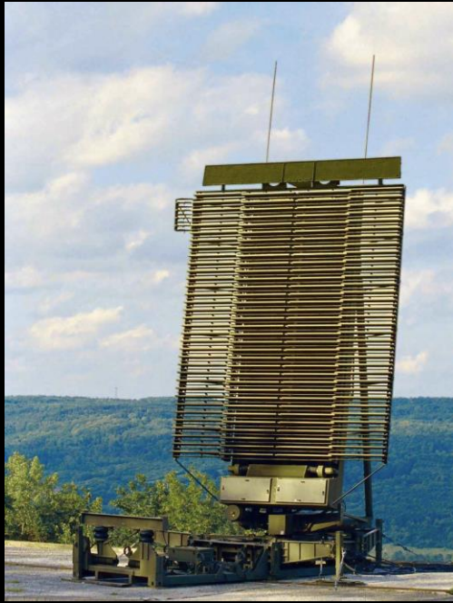
TPS-77 LR AIR DEFENSE RADAR Frequency – 1.2 to 1.4 GHz USA ORIGIN
