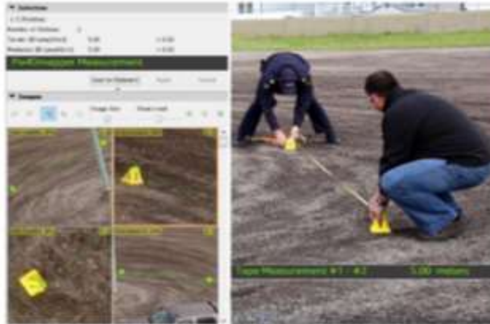
a) Compare UAV+Pix4Dmapper results with tape measurements
