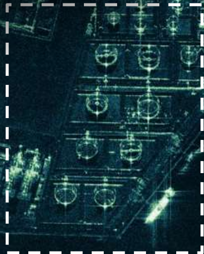
OIL TANKS OIL STORAGE LEVEL ESTIMATION
