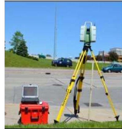
Terrestrial LiDAR system
