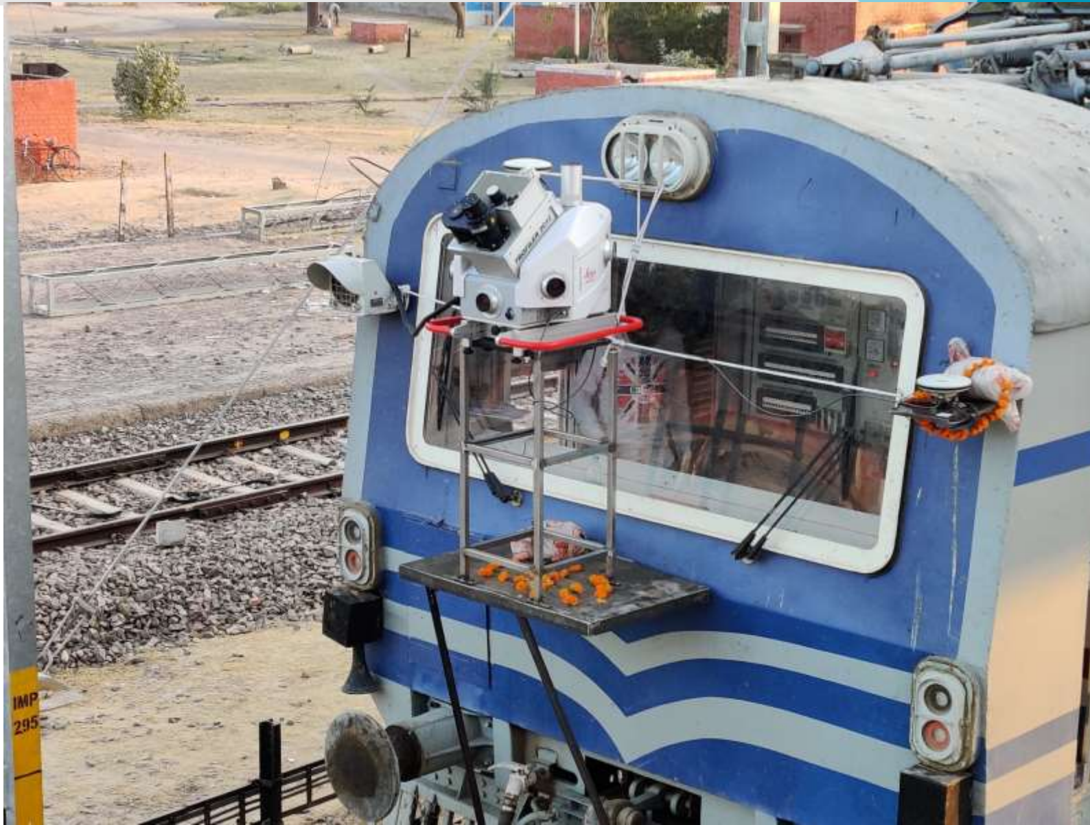
'Leica Pegasus Two' mounted on 'Tower Wagon' for Railway project :
