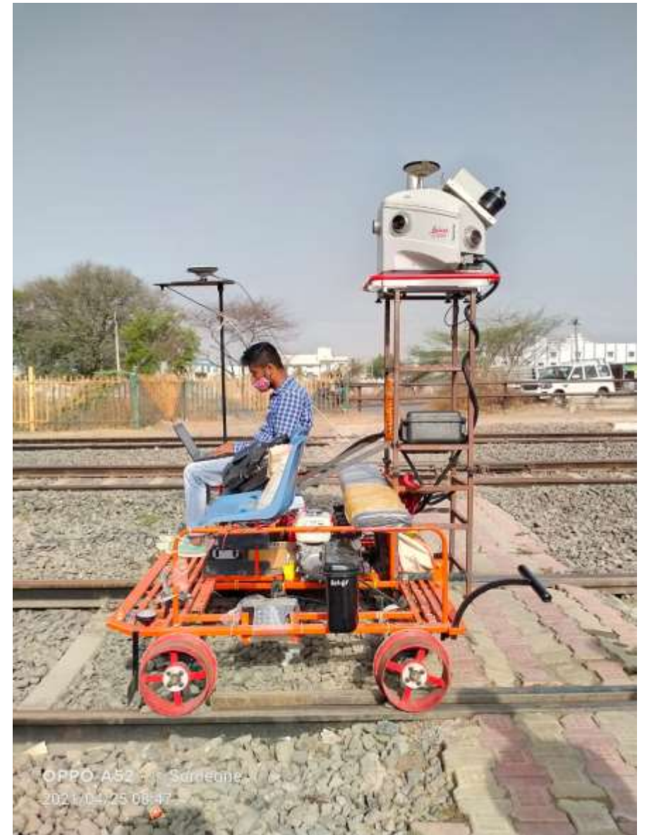
'Leica Pegasus Two' mounted on 'Motorized Trolley' for Railway project :
