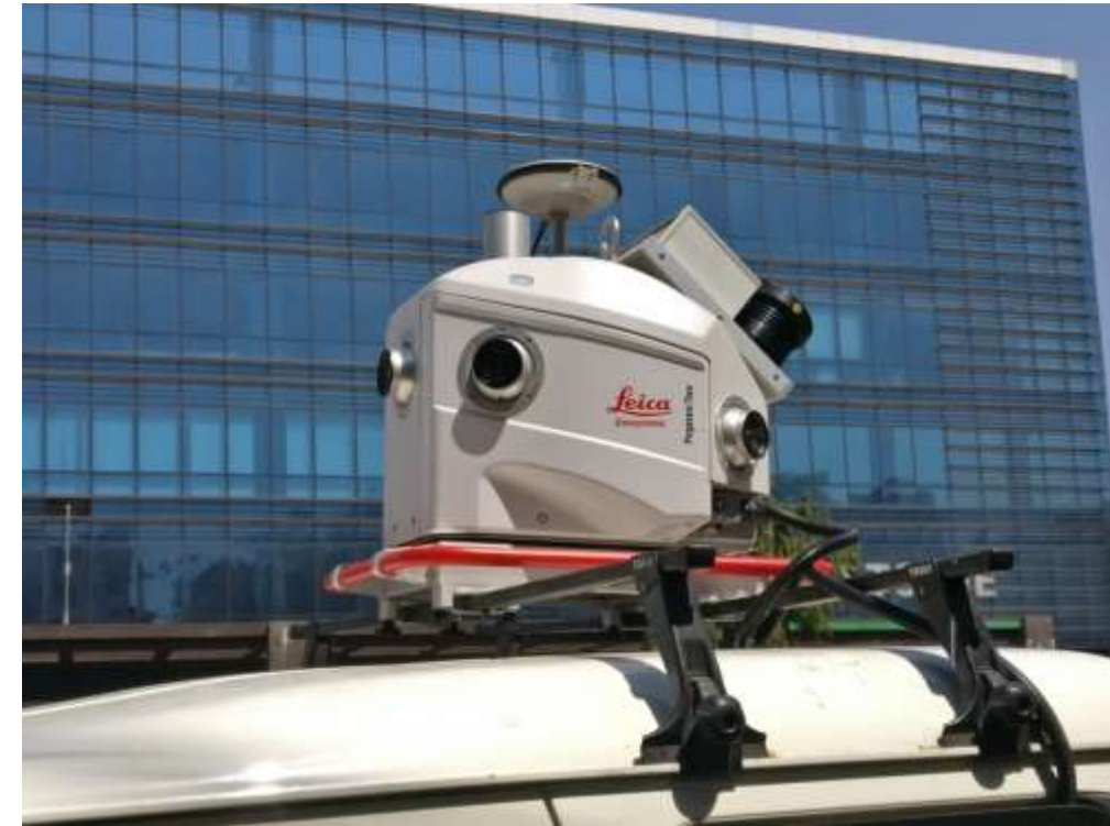
'Leica Pegasus Two' Mobile LiDAR mounted on a SUV vehicle.
